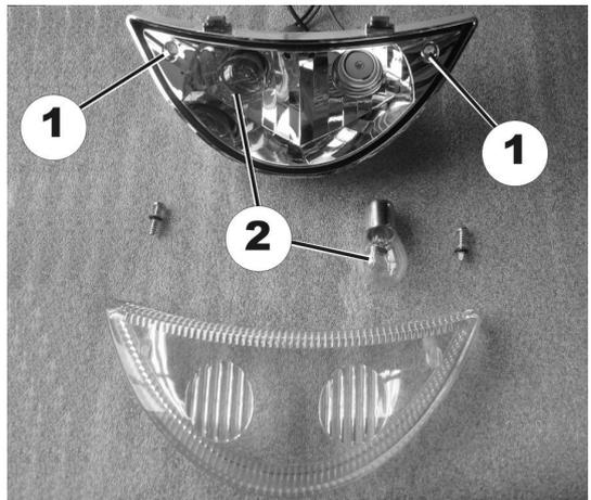
Remove screws (1) on headlight glass.
