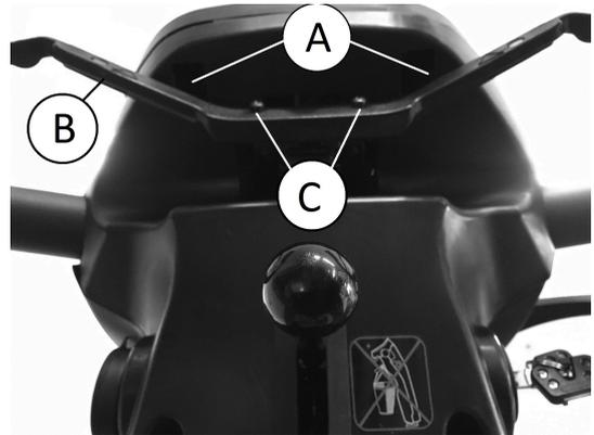
Remove screws (A) below operating console.
