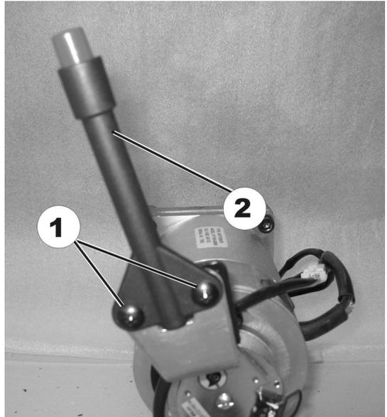
Remove screws (1) on disengaging lever (2).
