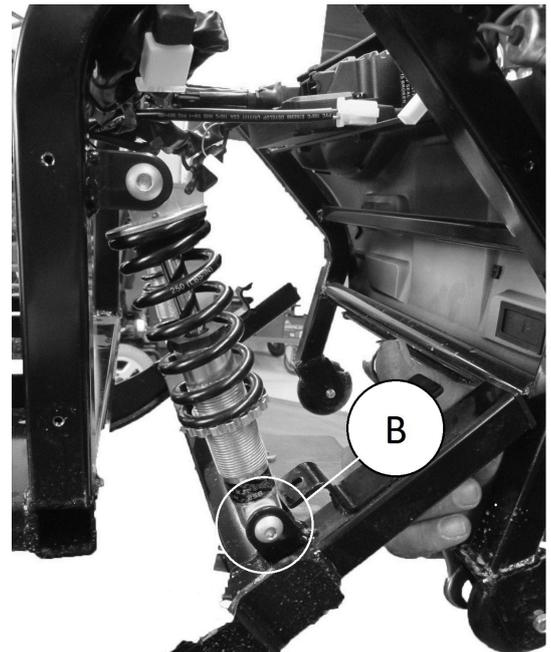
Loosen and remove lower bolt (B) on rear shock absorber on left and right side of the mobility device.
