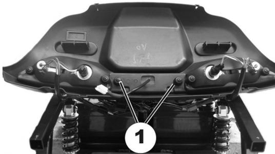
Remove screws (1) on brake light.
