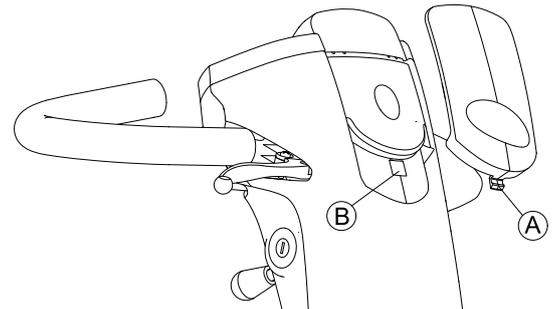
Remove top shroud (A) from steering column (B).
