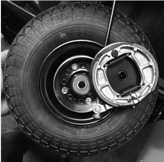
Pull brake out of brake drum.
