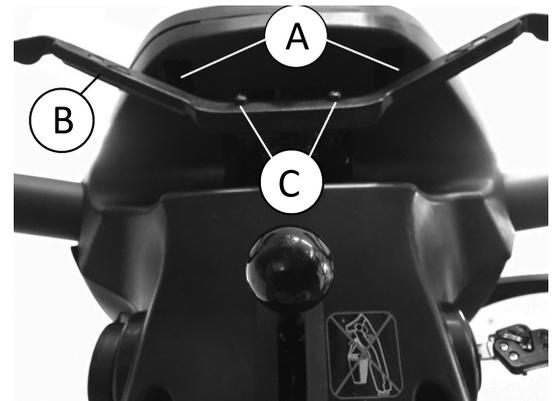
Remove screws (A) below operating console.
