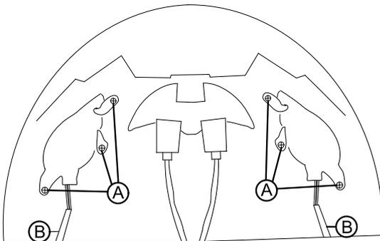
4. Disconnect direction indicator cable (B) from wiring harness.
