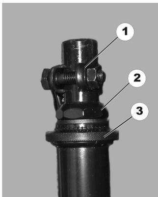
Loosen and remove screw at clamp (1).
