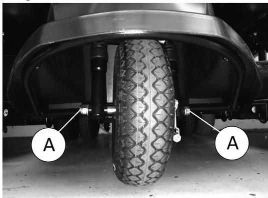
Loosen axle bolts (1) simultaneously on both sides.
