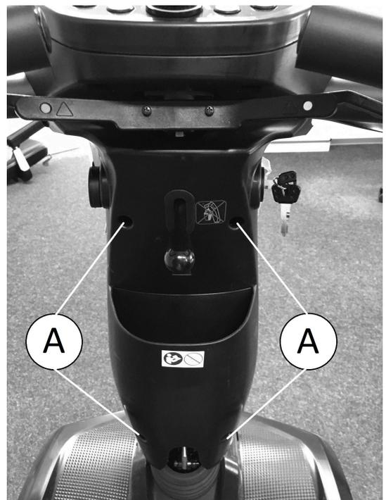
Remove screws Ⓐ on rear steering column shroud.
