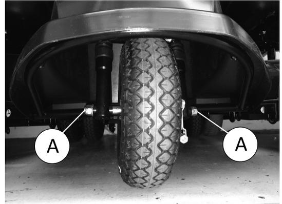
Place a supporting wooden block under the front part of the frame so that front wheel is no longer touching floor.
