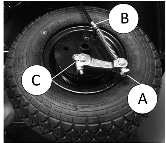
1. Slacken brake cable using setting screw **A**.
