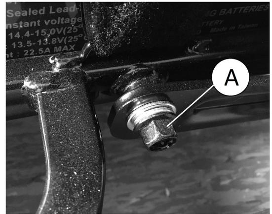
Loosen and remove screw (A) that attaches swing arm to chassis on left and right side of the mobility device.
