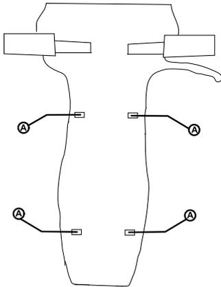
Remove screws **A** on front steering column shroud.
