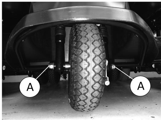
Loosen axle bolts **A** simultaneously on both sides.
