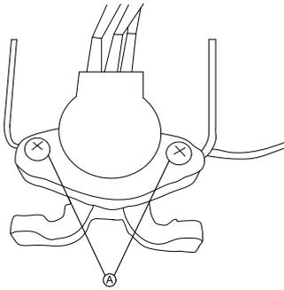
Remove screws **A** on potentiometer.
