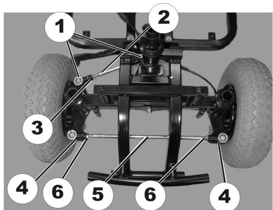
Remove circlip (1) on steering link (2).
