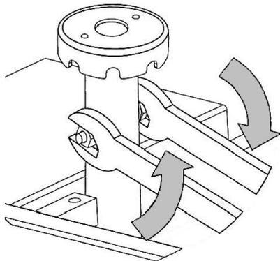
Loosen securing bolt of seat support tube.
