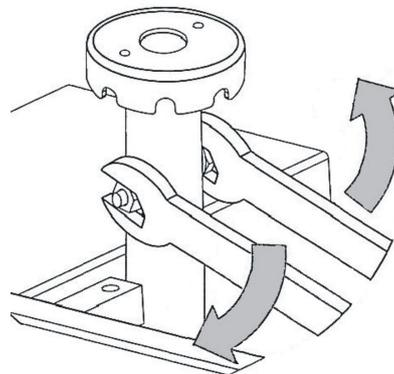
Firmly tighten securing bolt of seat support tube.
