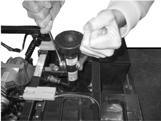
Remove securing bolt, nut and washers of seat support tube.
