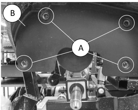
Remove screws (A) on mud guard.
