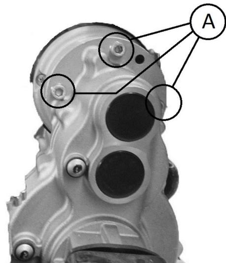
Loosen three Allen screws (A).
