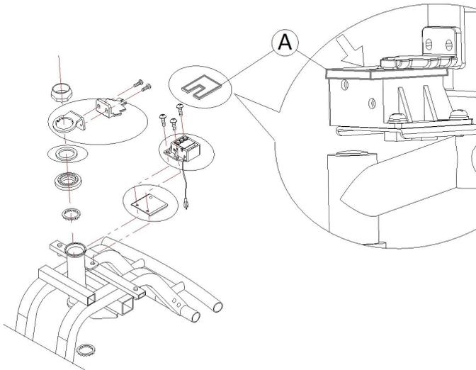
To check position of sensors of curve control device, use measuring gauge ① supplied in "Bend speed reducer retrofitting kit".
