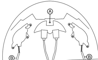
Remove screw (1) or ① on headlight under front shroud.
