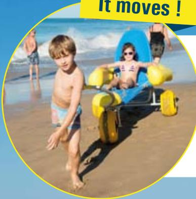
An accompanying person pulls and steers the three-wheeled chair with the help of a tow bar fitted with a handle. The low-pressure wheels make it easy to pull it over sand and pebbles.
